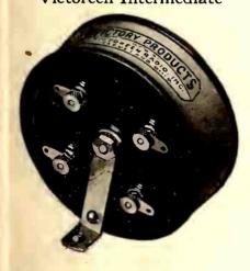
VICTOREEN intermediate transform-Walker Co., have a sharp resonance curve. This resonance feature of the coil permits use of an aperiodic primary, prevents interstage oscillation, makes the set more stable and permits the use of a potentiometer as a volume control.
