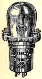
N interesting feature or the new A Mogul 5VC power amplifier tube put out by the Van Horne Co., and certified by Musselman, is an adapted base, in addition to the conventional tube base, on which are mounted four terminals for inclusion of higher B and C voltages than found in the normal sets without having to alter the wiring.
