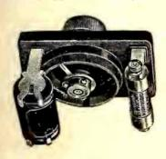
Two advantages noted in the use of changing the resistance are: ability to increase detector resistance to gain selectivity without losing energy transfer from antenna circuit, and to determine the degree of damping of the detector circuit in a reflex receiver, which damping may be made to aid regeneration.
